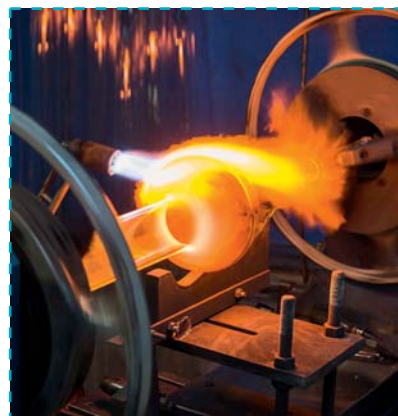
Glass tubes are blown by highly skilled blowers to ensure the excellent quality.
