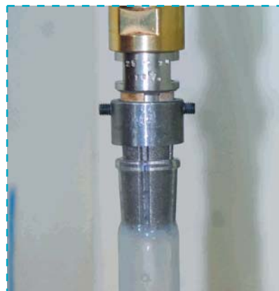
Grinding process of all joints performed by diamond reamers for best results.
