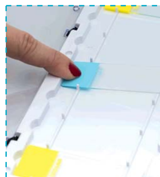
Removal of slides is done easily by pressing on one end, which will automatically lift the other end.
