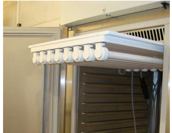
Easily removable and interchangeable lighting levels
