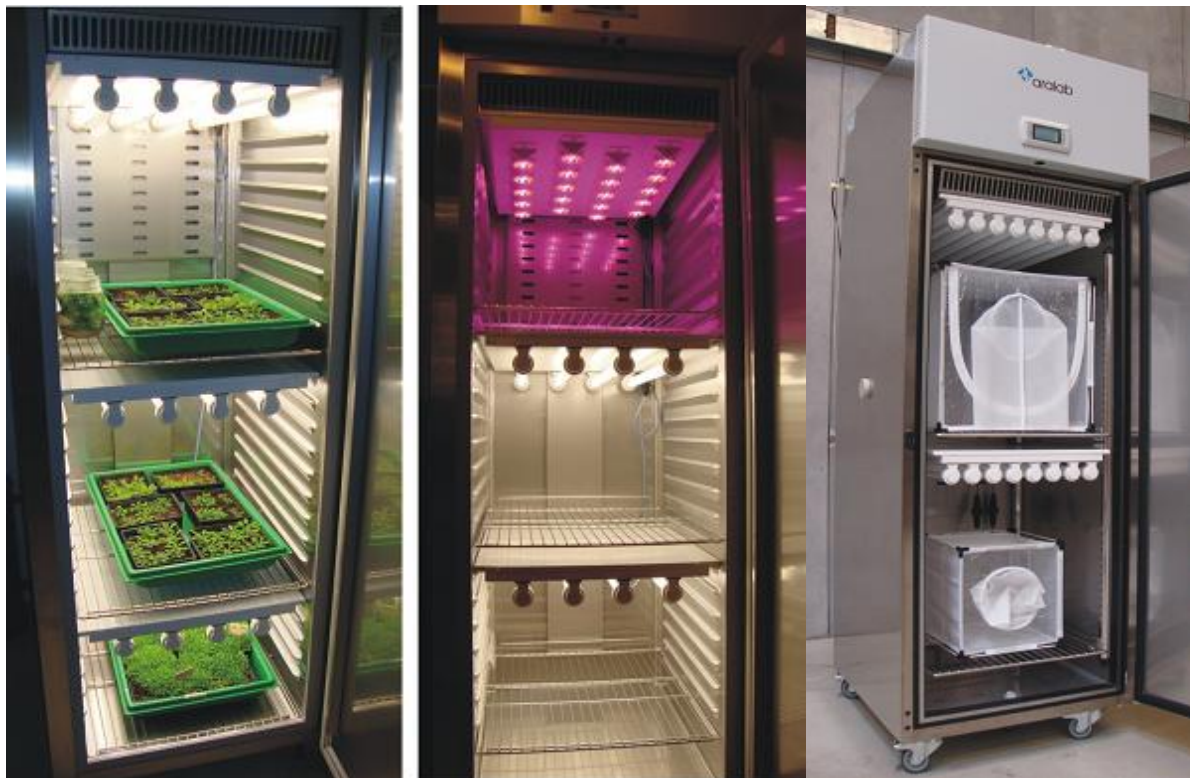
From left to right: S600PL with 3 lighting levels of 4 x 18W; S600PLH with 1 LED Grow Master (top) and 2 levels of 4 x 18W; S600 PLH with 2 shelves of 8x18W fluorescent cool white lights and entomology research nets on each wire shelf
